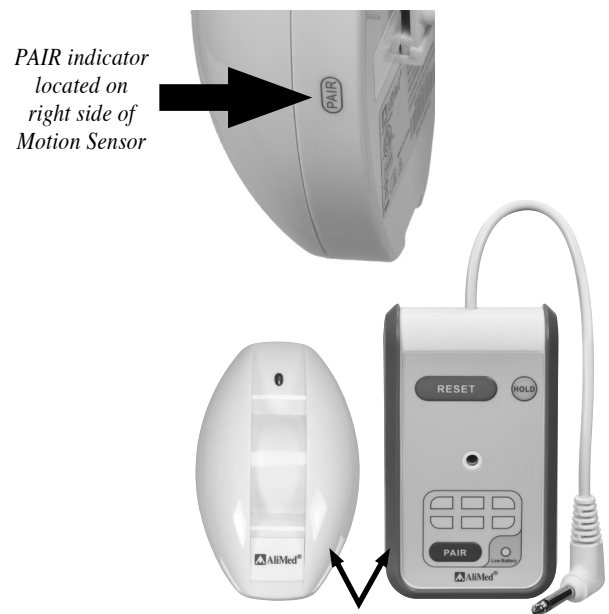
Match PAIR on Motion Sensor to PAIR on Base
